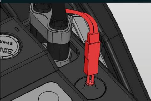
If the cable isn't connected properly, the display will show a -40 C readout under the speedometer.
